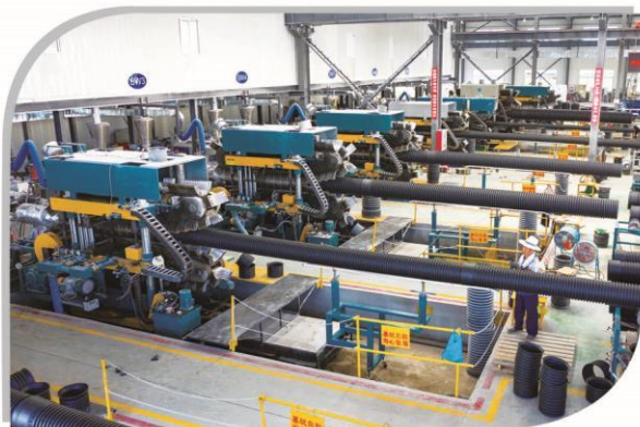
HDPE双壁波纹管生产车间
